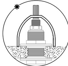
\* Adjust valve height using the JIG as shown
