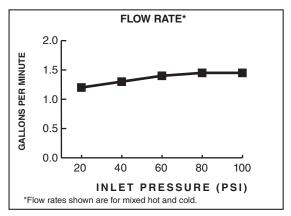
1.5 gpm/5.7 L/min. FLOW RATE
