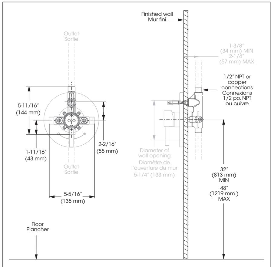
Valve – Rough-In // Pressure Balanced Diverter Valve with Volume Control
