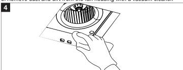
4. Dampen cloth with dish detergent, wipe the fan housing and dry with a cloth. Replace the grid.
