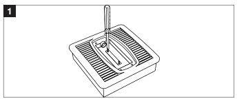
1. Remove the grille by unscrewing the screws, then pulling the grille down.
